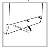
1. 以螺絲批鬆開機前部擋板(見圖) using a screwdriver, remove the cover panel on the lower front part of the washer-dryer (see figure).
